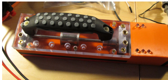
v1 - 3D-printed housing, acrylic top plate, brass inserts and drive coil.
